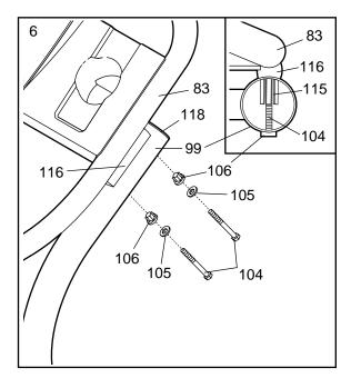
7. Make sure that all parts are properly tightened before you use the treadmill. Keep the included allen wrench in a secure place. The allen wrench is used to adjust the walking belt (see page 27). To protect the floor or carpet from damage, place a mat under the treadmill.
